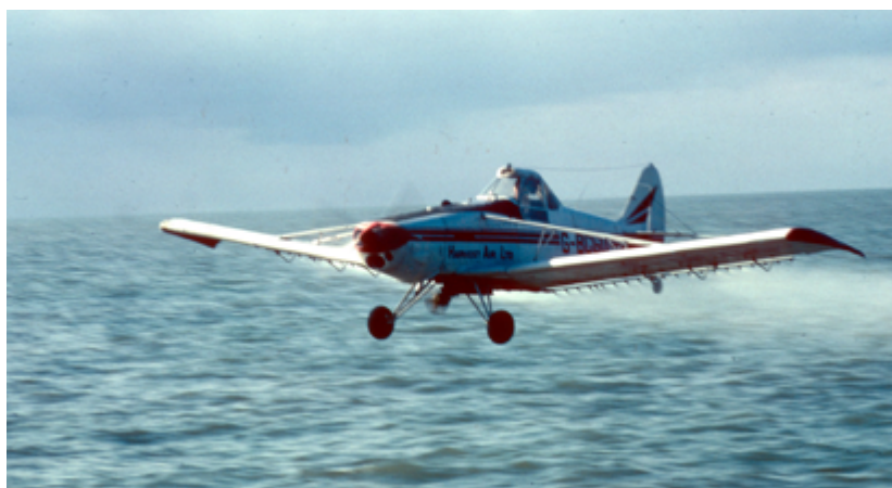
Figure 2 – Converted crop-spraying aircraft applying dispersant during the Betelgeuse oil spill. (Source: ITOPF)
