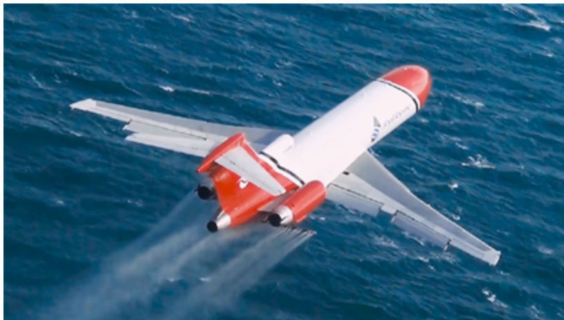
Figure 23 – Boeing 727 equipped with purpose-built pump systems and storage tanks. (Source: OSRL)
