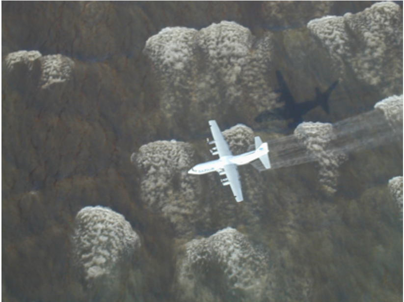
Figure 29 – Dispersant spraying operation performed with a large multi-engine aircraft. (Source: ITOPF)
