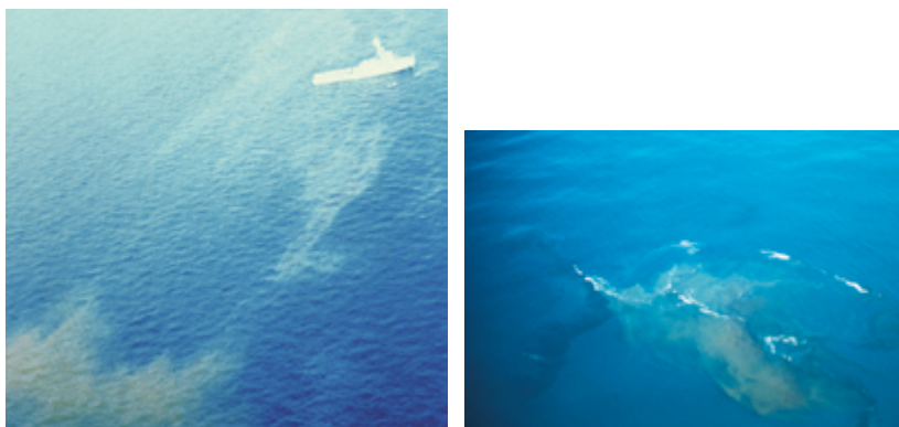
Figure 53 – What the pilot sees: plume of dispersed oil (brown/beige) appears quite distinct from the surface oil (which is black or metallic). Note the presence of cloudy/white patches in some areas, which indicates that too much dispersant may have been sprayed or that targeting was inaccurate. (Source: CEDRE)
