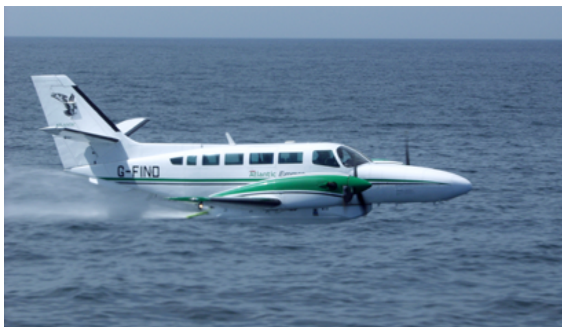
Figure 22 – Medium-size aircraft equipped with a pod designed for dispersant application. (Source: CEDRE)
