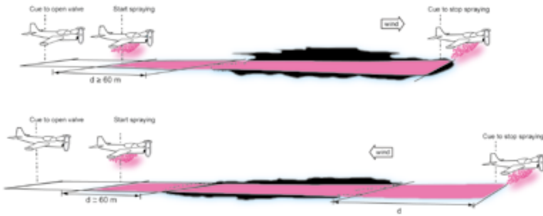
Figure 40 – Spraying dispersant on the sea surface: spray downwind, spray upwind. (Source: CEDRE)
