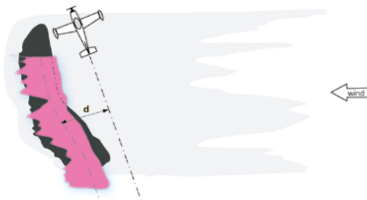
Figure 39 – Aircraft flying in a crosswind direction to treat a strip of oil. (Source: CEDRE)
