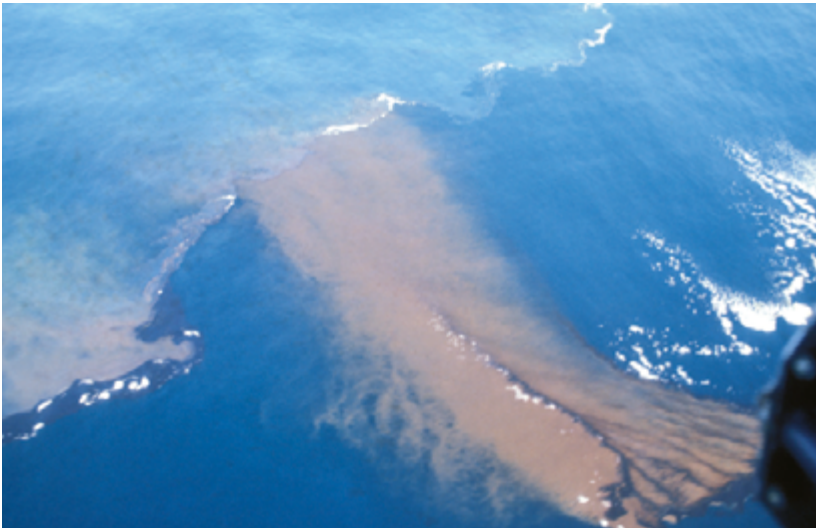
Figure 51 – When the wave goes through the treated slick, the additional agitation assists by placing the oil in suspension and the brown plume of dispersed oil forms. (Source: CEDRE)
