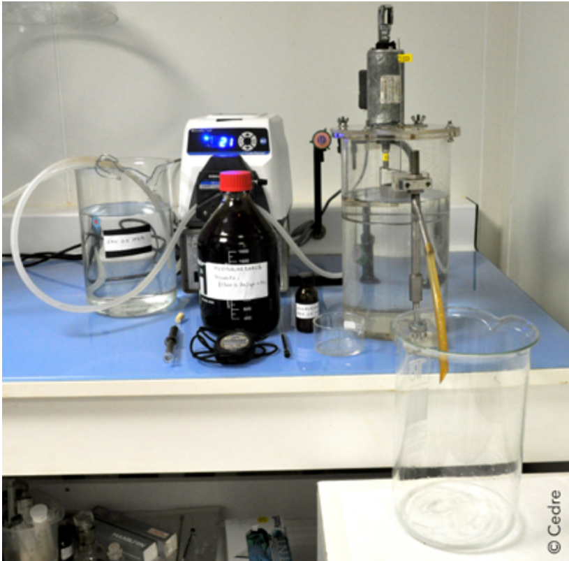
Figure 18 – Dispersant effectiveness laboratory test method: IFP flow-through test used in France. (Source: CEDRE.)
