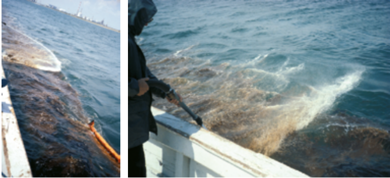
Figure 50 – Dispersion trial. Note the brown colour of the plume immediately after spraying. (Source: CEDRE)
