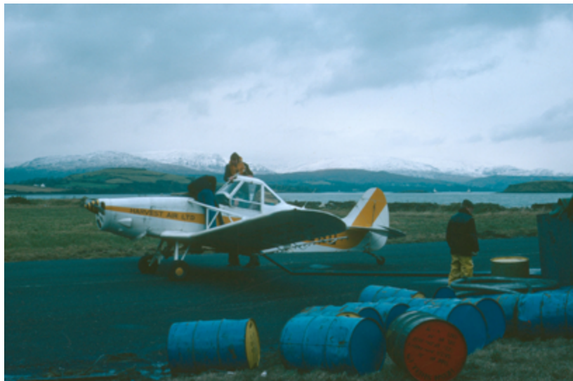
Figure 26 – Refilling dispersant on a small crop-spraying aircraft ( Betelgeuse oil spill). (Source: ITOPF)
