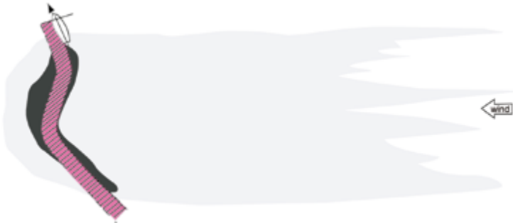
Figure 49 – Application procedure when the oil is gathered in strips across the wind. (Source: CEDRE)
