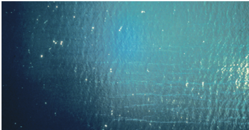
Figure 58 – The same slick a day after being sprayed. The dispersion plume has dissolved into the background. All that is left is sheen which is waning and disappearing. (Source: CEDRE)
