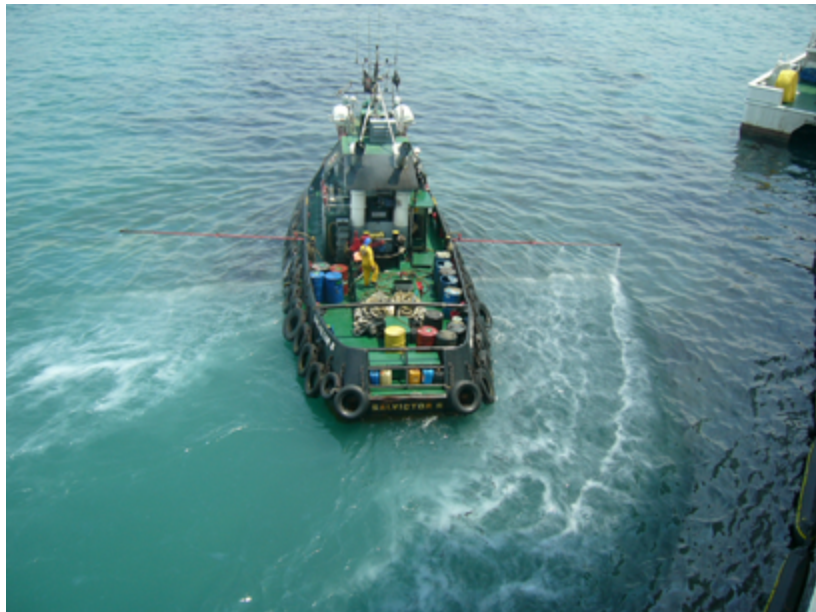
Figure 24 – Dispersant application from a tugboat. (Source: ITOPF)
