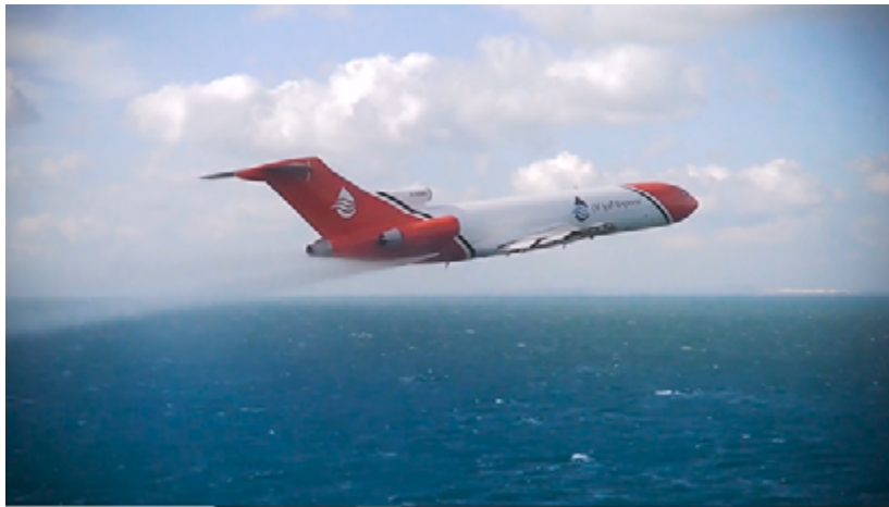
Figure 1 – Large aircraft (Boeing 727 with Tersus system) completing a spraying exercise operation. (Source: OSRL)
