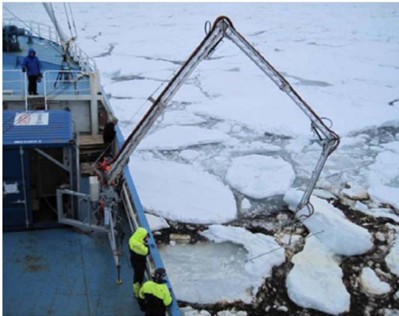
Figure 17 – Dispersant application using a remote-controlled spray boom in the icy Arctic environment. (Source: SINTEF)
