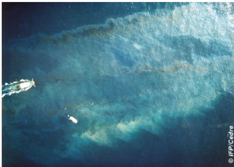
Figure 6 – Oil slick at sea treated by a ship performing parallel spray runs during sea trials. (Source: IFP/CEDRE)
