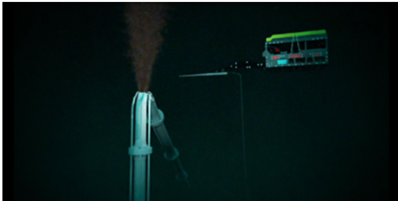
Figure 62 – Subsea dispersant injection into a broken riser. (Source: Wild Well Control)
