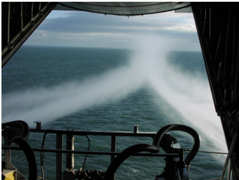
Figure 21 – View of the spray pattern seen from the inside of a large aircraft (C-130 Hercules). (Source: ITOPF)
